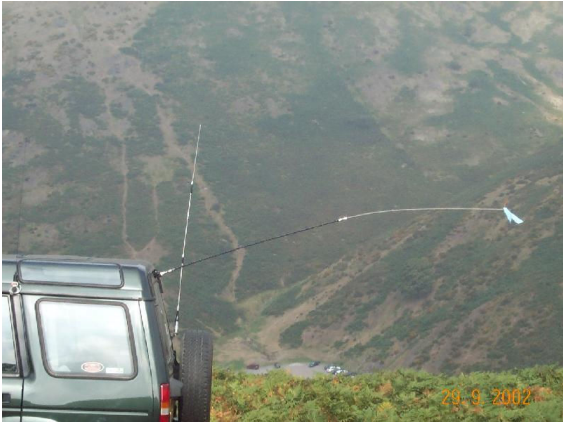
Figure 1. The NVIS mobile installation used for the Longmynd Hike by M5WJF/M. Note the deliberately horizontal whip designed to optimise F2-layer near-vertical reflection back down into neighbouring valleys.
